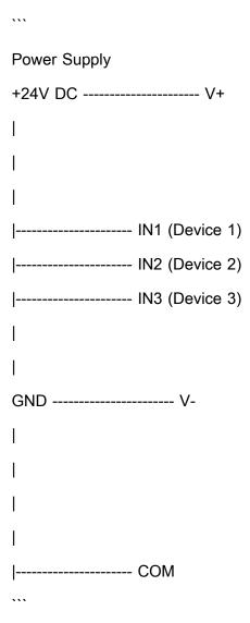
This diagram illustrates how the power supply connects to the module and how individual devices
